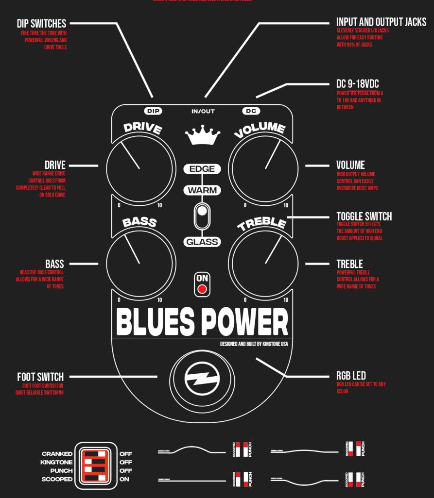
CRANKED BOOSTS THE SECOND OVERDRIVE STAGE TO GIVE A CRANKED AMP TYPE OF TONE KINGTONE CHANGES THE OVERALL VOICING OF THE PEDAL TO PROVIDE MORE BITE AND FATNESS PUNCH & SCOOPED CONTROL THE MID RANGE OF THE PEDAL
